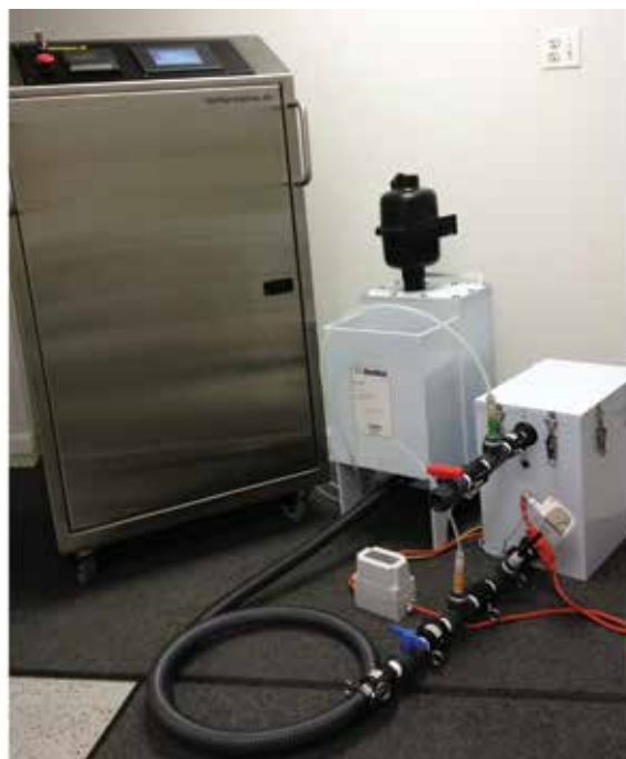
Figure 1. Decontamination equipment, using a Minidox-M Decontamination System (ClorDiSys Solutions).
