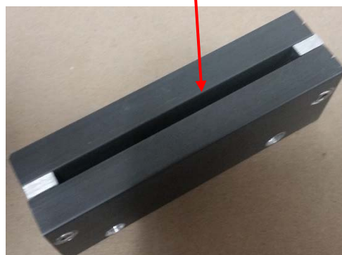
Figure 2: BI Challenge Fixture. This is a test fixture to mimic small gaps. BI is placed into the small opening or slot to test the penetration of CD gas into small gaps or openings. Simulates a 5mm gap.
