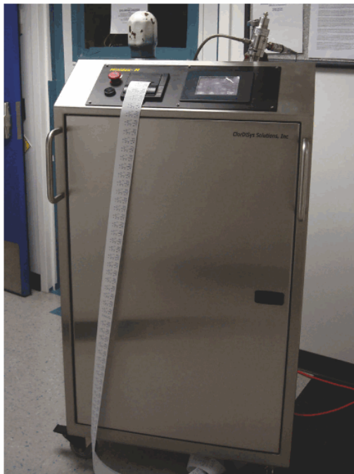
The Minidox - M Decontamination System provides a rapid and highly effective method to decontaminate a target chamber. The system features a sophisticated sterilant concentration monitoring system to assure a tightly controlled decontamination process.
