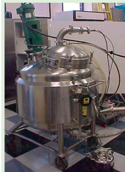
Photo 3: 500-liter pharmaceutical process vessel
