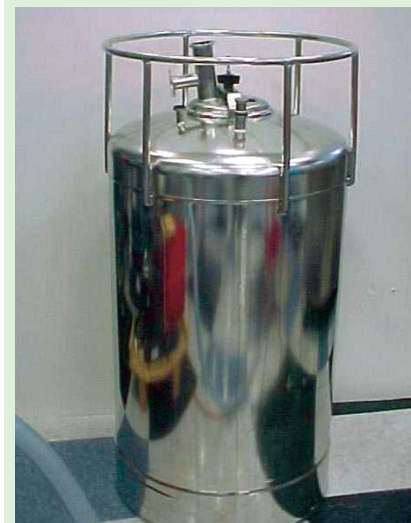
Photo 2: 100-liter pharmaceutical process vessel
