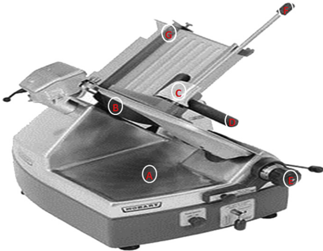
Fig. 1. Different selected sites inoculated with L. monocytogenes cocktail on the commercial meat slicer. A: SS base; B: blade; C: SS grip; D: plastic handle; E: plastic handle; F: plastic handle; G: SS removable carriage.
