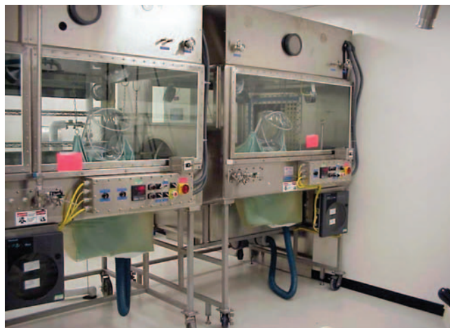
Figure 4: A train of isolators (total 279 ft 3 ): a workstation isolator (a 150-ft 3 316 SS workstation isolator with 2 half suits, 6 circulation fans, high-efficiency particulate air [HEPA] filters, and a pressure blower), an autoclave interface isolator (a 90-ft 3 316 SS workstation isolator with 1 half suit, 4 circulation fans, HEPA filters, pressure blower, and pressure control [disabled in interface isolator]), and an autoclave (a 39-ft 3 316 SS autoclave). Total cycle time is 2 h.
