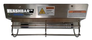
The 2-bulb, 4 foot Flashbar outputs UV-C light at 68 µW/cm<sup>2</sup> at ten feet to provide disinfection of surfaces in minutes.
