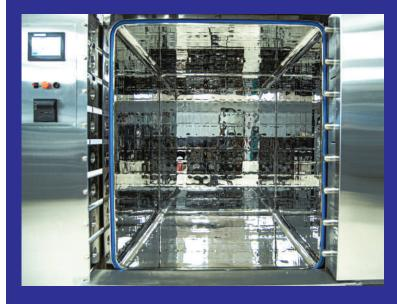
Chlorine Dioxide Sterilization chambers range in size to conform to capacity needs, currently up to four pallet loads. Due to the simplicity of the sterilization process, every step including; conditioning, exposure, and aeration, all occur within the chamber. Cycle times are also significantly lower in most scenarios.
